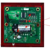
When the low battery signal is received at the 1117 RX master the battery will have to be changed to stop the low battery beep
